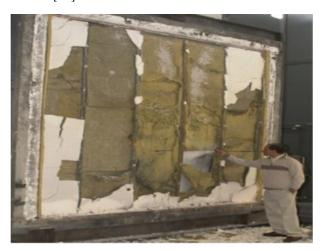
b) Post fire inspection of test wall
